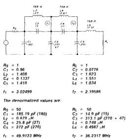
tune  $L_2$ ,  $C_2$  for an attenuation peak at  $f_1$  tune  $L_4$ ,  $C_4$  for an attenuation peak at  $f_2$
